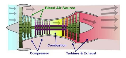
Figure: shows air entering the front of the engine where a series of turbines compress, warm and pressurize the air before it passes into the combustion chamber where it is ignited to create the airplane's thrust. This "bleed" air is drawn out of the engine into the cabin after it is pressurized, but before the combustion chamber.
