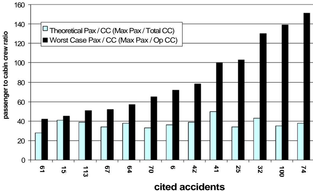
Figure 2: Comparison of Theoretical Ratio and Worst Ratio in the 13 cited accidents in which the Worst Ratio
