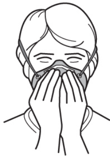
Figure 5: Seal check with a disposable respirator
