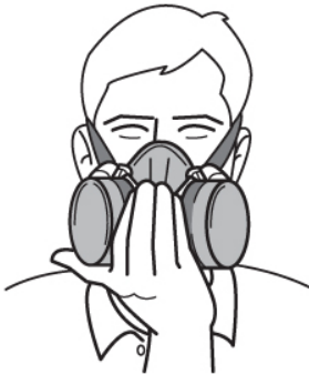
Figure 4: Positive pressure fit check
