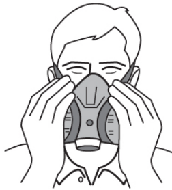
Figure 3: Negative pressure fit check
